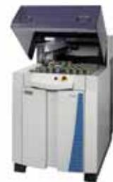
ARL Perform'X X射线荧光光谱仪 (WDXRF)
