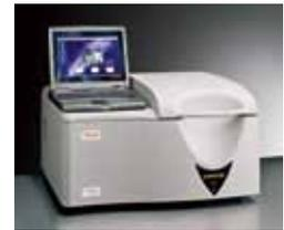
ARL Quant'X X射线能谱仪 (EDXRF)
