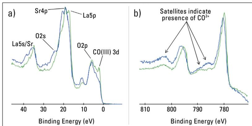
Figure 7: a) Valence band spectra and b) High resolution cobalt spectra from as received and annealed LSC surfaces (0-6 nm)
