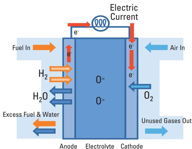
Figure 1: Schematic of operation of solid oxide fuel cell
