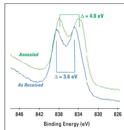
Figure 5: High resolution lanthanum spectra of the surface
