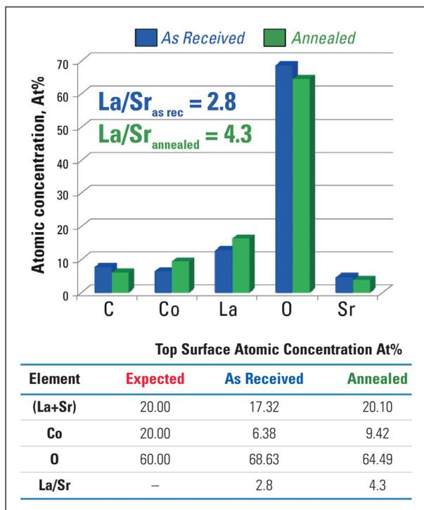
Figure 3: Elemental quantification of surface composition of annealed and as received samples
