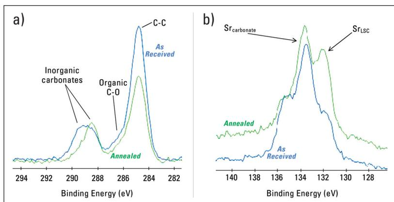
Figure 4: High resolution spectra of a) carbon and b) strontium
