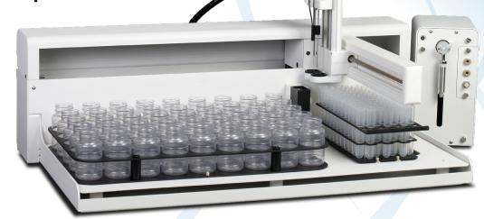
Pre-analysis preparation of oil samples is achieved via a relatively simple dilution process. Manual dilution is time consuming, labor intensive and carries the potential for human error. Eliminate all of these concerns with this high throughput dilution system for oil samples
