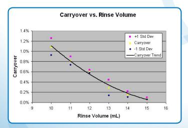
Customizable rinse volume setting determines percentage of carryover with typical carryover of less than 0.2%.
