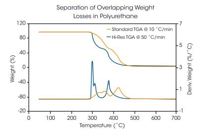
The figure above shows the Hi-Res TGA results for a polyurethane material by standard and Hi-Res TGA. The superior resolution provided by the Hi-Res technique is clearly evident in both the TGA weight loss and the first derivative (DTG) signals. The latter signal is especially useful in defining the onset and the end-set of the individual weight loss segments, as well as indicating subtle events that provide a "fingerprint" of the sample.
