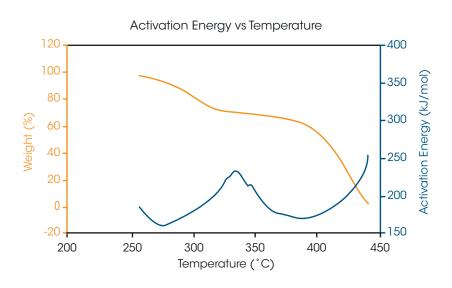
TA's patented MTGA\* is another TA Instruments innovation that offers advantages for material decomposition studies. Developed from the proprietary heater control technology utilized by Hi-Res TGA and MDSC, MTGA produces model-free kinetic data. Activation energy can be calculated real-time and studied as a function of time, temperature, and conversion.
