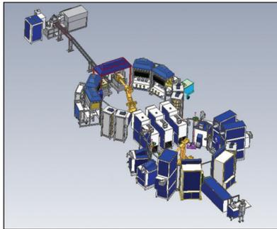
**Line for sample preparation and OE analysis allowing a throughput of 1000 samples a day.\***
