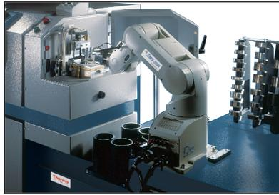
**The lead button is automatically transported on a belt conveyor to the ARL SMS-2000. The button is automatically weighed on an electronic balance, surfaced in an automatic milling machine and finally analyzed with the ARL Fire Assay Analyzer.\***
