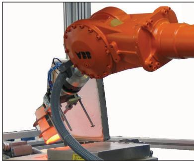
**Separator furnace: the melt obtained in the fusion furnace is poured by the handling robot into a furnace holding a heated separator crucible for the separation of the metallic lead and slag.\***
