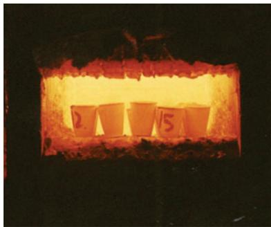
During cupellation, the Pb is oxidized by the air and mostly absorbed by the cupel, leaving only a PM bead or prill, which is further analyzed by various techniques, according to the particular analytical requirement, e.g:
